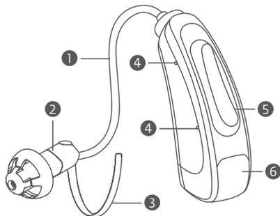
☞ The hearing aids have markings for the sides on the receiver module: blue = left, red = right
