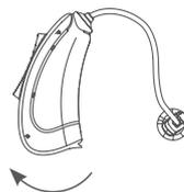
Open the battery compartment carefully with your fingernail at the edge for opening and swing it right out.
