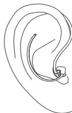
The optional Concha-Clip helps improve the fit of the receiver unit in the ear. To position the Concha-Clip, bend slightly and place the Concha-Clip carefully in the outer part of your ear.
