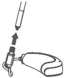
Pull out the filter with a gentle turning motion.
