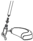
Press the new filter with the changing tool into the filter opening of the hearing aid until it clicks into place. Then simply pull out the replacement tool and dispose of it.
