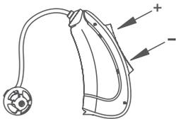
The volume can be adjusted in steps using the multifunctional rocker switch. Briefly pressing the top end of the switch increases the volume, while briefly pressing the bottom end reduces the volume.
